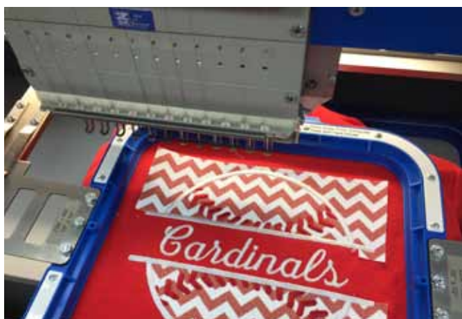
The third and last step is the finished edge, typically a solid satin stitch, that covers the exterior of the raw fabric.
